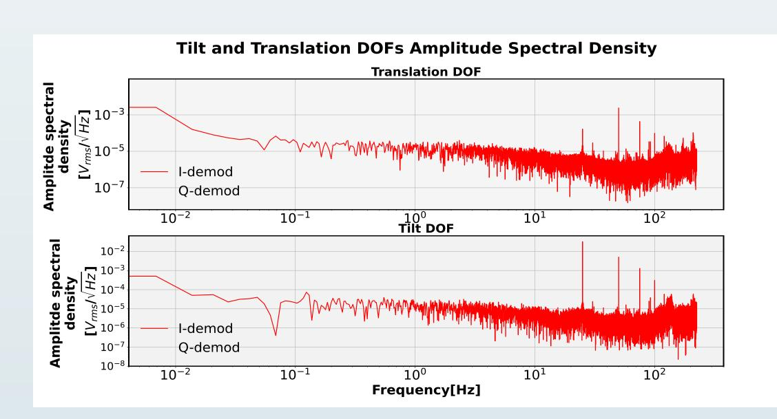
Amplitude Spectral Density: Above is the amplitude spectral density while driving each DOF at 25 Hz. In the graph below we normalize\* the spectral density with respect to the misalignment coupling coefficients  $\frac{a}{\omega_0}$  and  $\frac{\alpha}{\Theta_{mod}}$  at each demodulation. The sensed DOF's noise is about 10-100 times better than the not sensed DOF.
