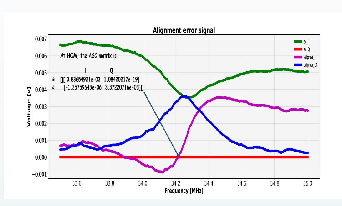
Alignment Signal: Frequency sweep of the alignment error signal matrix. We expect when we drive the EOBD at the HOM frequency, we get a well-separated alignment signals, and that's what we see here, at the right frequency and demodulation phase we get a diagonal sensing matrix.
