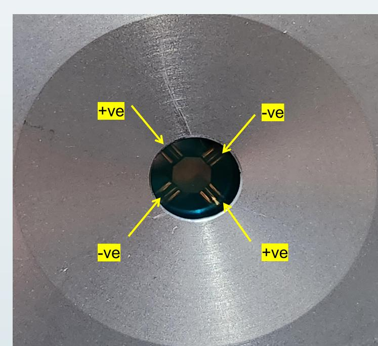
**EOBD:** We see the octagonal Lithium Tantalate ( $LiTaO_3$ ) crystal that is used to deflect the beam. Voltage is applied to the 4 electrodes, creating timedependent  $\vec{E}$  inside the crystal that changes the refractive index.
