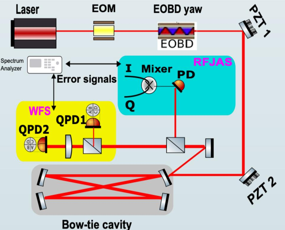
**The current setup:** We have a laser, then EOM for the PDH locking and WFS, EOBD for the alignment, PZTs to drive DOFs, and then the cavity. On reflection we have two PDs. One for PDH signal and the other is the single element PD to generate RFJAS signals. Gouy phase telescopes are after that for WFS signals.
