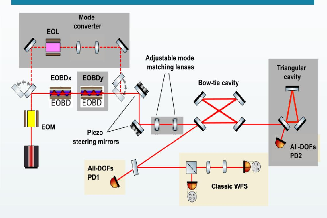
**Future Work: upper diagram** shows the future work that could be implemented on our table-top experiment at UF. In gray boxes are the components and optics that are not currently set up. That includes Electro-Optic Lens (EOL) to generate alignment signals for modemismatch, and any 2<sup>nd</sup> order HG errors, and a 2<sup>nd</sup> cavity on transmission.
